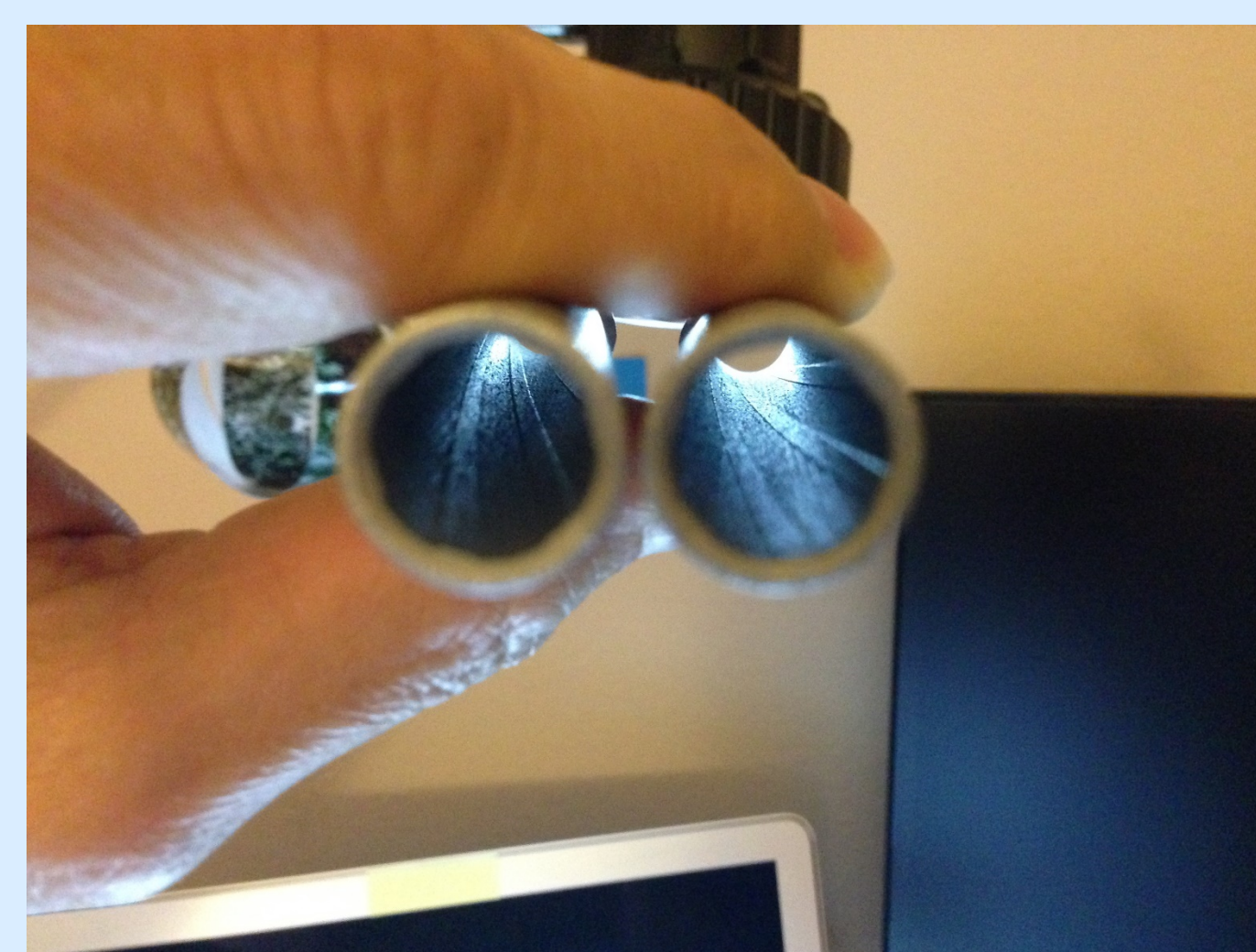
Figure 2: Two identical 3D printed gun barrel
